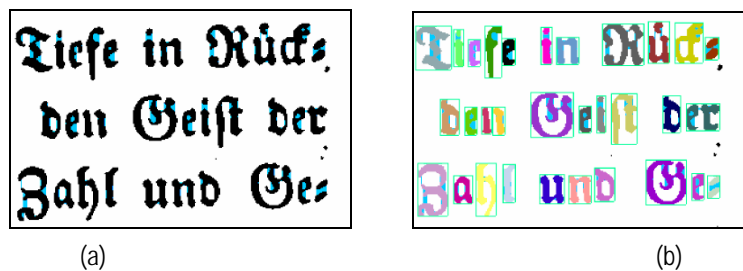
Figure 4. Example of applying RLSA. (a) result after smoothing; (b) character segmentation result.
