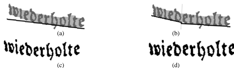
Figure 28: Example of baseline estimation and rotation of a distorted word; (a) initial baseline estimation; (b) baseline estimation after word has been splitted; (c), (d) rotation of the word using the baseline of (a) and (b), respectively.
